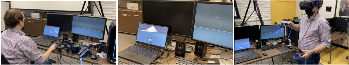
Figure 1: Single-user CR prototype for reservoir engineering data visualization. The user performing analytical work on a laptop transit 3D reservoir model from standard monitor to VR space to increase working space and improve spatial perception.
