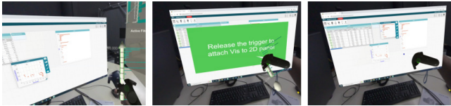
Figure 2: The process of “pushing” a visualization into a 2D monitor panel. From left to right: 1) before pushing the Axis into the panel, 2) colliding the Axis with the virtual representation of the monitor and seeing the release prompt, and 3) releasing the Axis and the creation of a visualization on the desktop side.
